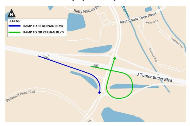
FDOT hired J.B. Coxwell Contracting to complete the \$17.1 million project, which includes construction of a partial cloverleaf interchange, adding capacity to on- and off-ramps, milling and resurfacing of existing pavement, roadway lighting improvements, construction of ponds and other drainage improvements and installation of new signage and mast arm signals. The project is estimated for completion in late 2024, weather and unforeseen circumstances permitting.
